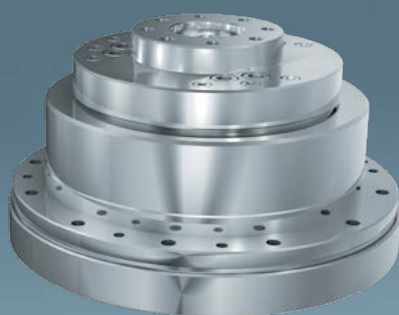
GH Solid shaft T: 69–980 Nm i: 10.74–31.43 n: up to 270 rpm
